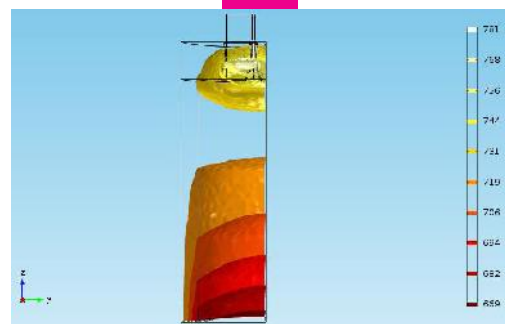
Image 8: Isothermal billet temperature change displayed in COMSOL on the y-z plane
