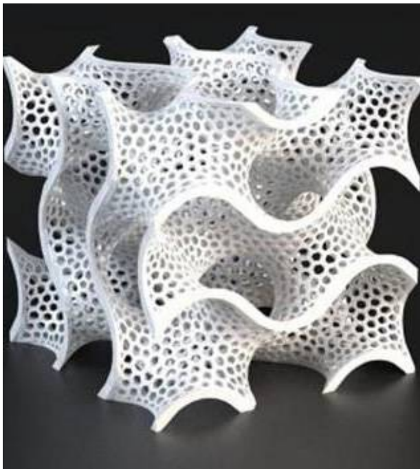
Figure 13. Highly detailed sculpture manufactured by SLA
