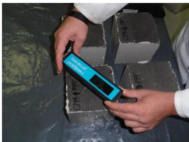
Image 4: Measuring electrical resistivity with a Resipod instrument
