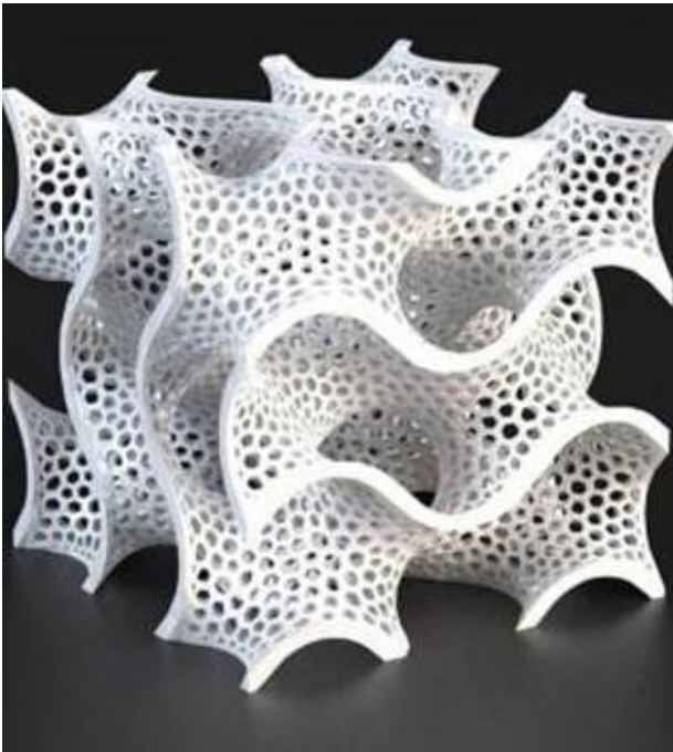
Figure 13. Highly detailed sculpture manufactured by SLA
