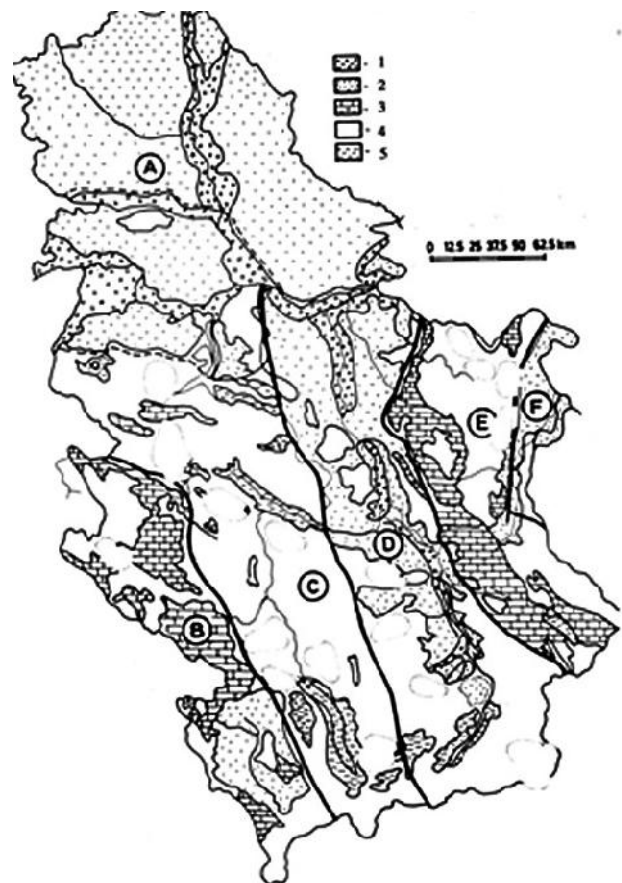
Figure 2. Geotectonic units of the territory of Serbia. A. Pannonian basin, B. Dinarides of Western Serbia; C. 22 Vardar zone; D. The Serbo-Macedonian mass; E. Carpatho-Balkanides; F. Dakian basin; 1. Alluvial formations; 2. Neogene lacustrine sediments; 3. Limestones; 4. Fractured formations; 5. Neogene clay sediments
